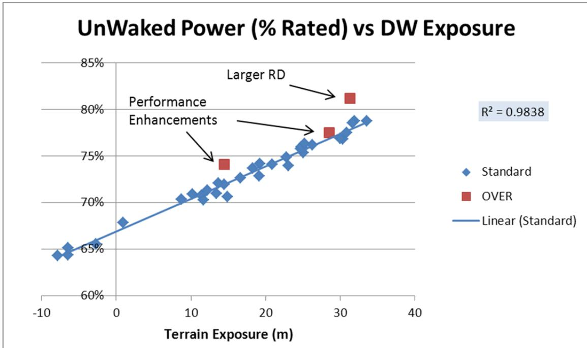
The turbine with the larger rotor has an average power that is clearly well above the trend established by the 33 standard turbines and the two with the blade enhancements have average power above the trendline. It is noted that the data set in this analysis includes data records before the performance enhancements were added, so their effect is not indicated as clearly as when the data are filtered again by time to include only data records when the enhancements were in place.
