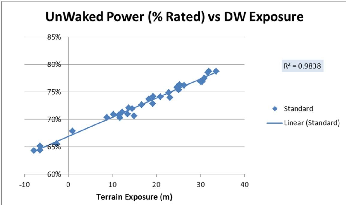
In that analysis we observe a very highly correlated relationship between the average power for the same 33 turbines and their downwind exposures. This clearly indicates that, indeed, the downwind terrain has a huge impact on how fast the wind blows, and, perforce, how much power the turbines will produce.
