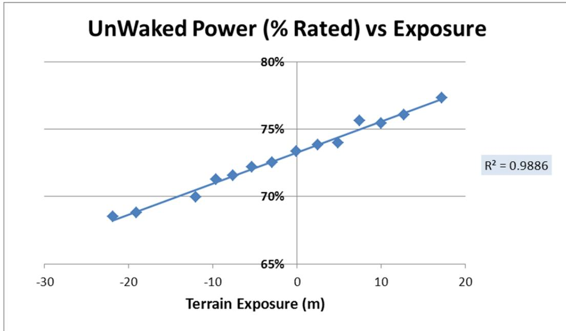
Once again a very high level of correlation was achieved between terrain exposure and turbine power. This shows that at this site, as well, the wind, which produces the observed turbine performance, is directly influenced by terrain, which was characterized by the exposure calculated with the RAMWind model.
