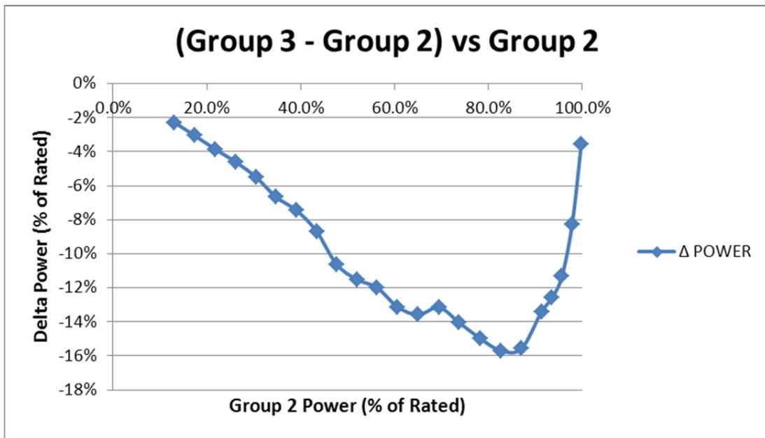
In the case of turbines that appear to be performing properly, but have a less-energetic wind resource, the relationship is quite regular and consistent up to the point where Group 2 is producing at approximately 85% of rated power. Above that power level Group 2 is
