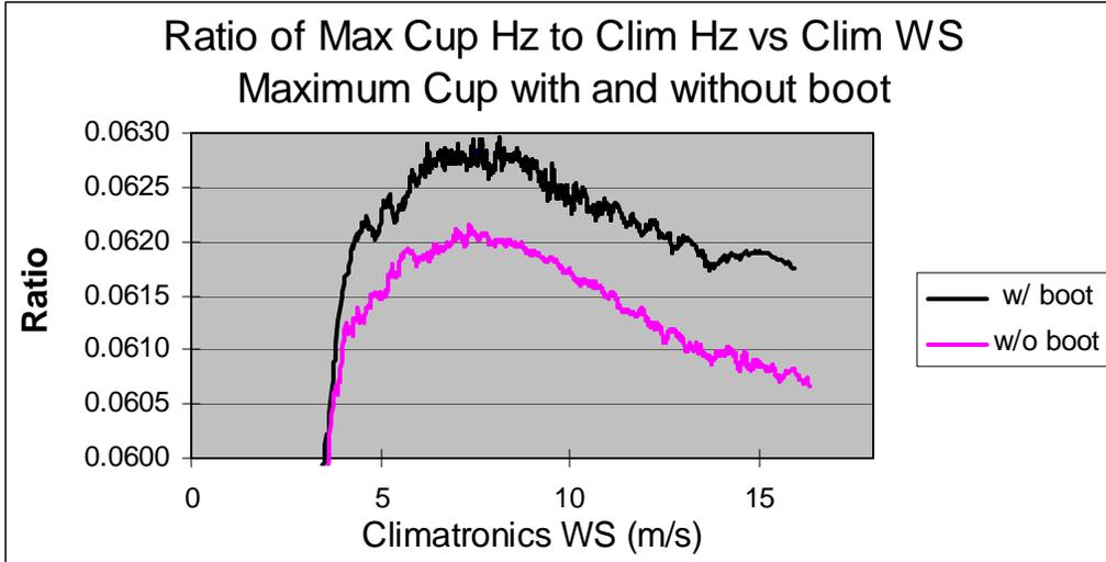
Figure 4. Comparison of rotational speed of old, used Maximum Cup and new Maximum Cup to Climatronics.
