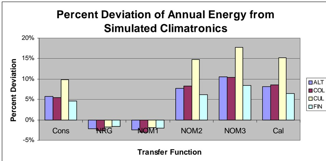
Figure 5. Percent deviation in theoretical energy from simulated Climatronics for different Maximum Cup transfer functions.
