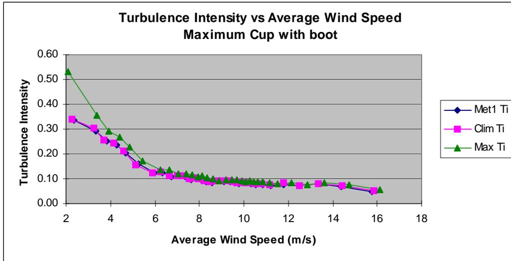
Figure 3. Ti versus wind speed for all three sensors.
