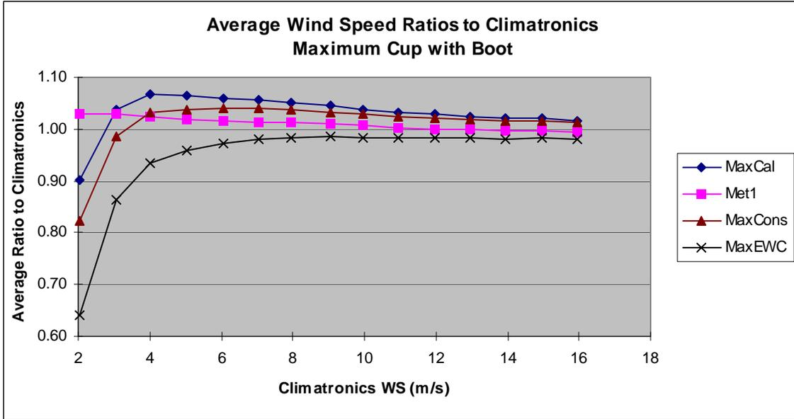
Figure 1. AVERAGE WIND SPEED RATIOS TO CLIMATRONICS WIND SPEED AS A FUNCTION OF CLIMATRONICS WIND SPEED.
