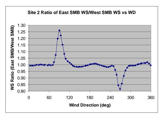
FIGURE 1. SMOOTHED RATIO (EAST SMB/WEST SMB) OF AVERAGE WIND SPEED AT SITE 2 EAST SMB/WEST SMB VERSUS WIND DIRECTION.
