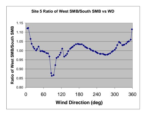
FIGURE 2. SMOOTHED RATIOS (WEST SMB/SOUTH SMB) OF AVERAGE WIND SPEED AT SITE 5 VERSUS WIND DIRECTION.
