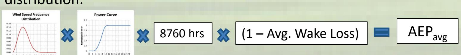
2) Then, the AEP was estimated assuming that the ratio of night/day wake loss = 2.0 and using wind speed distributions representative of daytime and nighttime conditions
